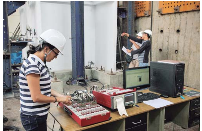
Staff measuring the earthquake damage to a wall (Photo: Kosuke Okahara /JICA)
